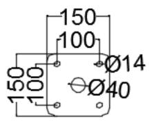
\*Measurements in millimeters (mm)
